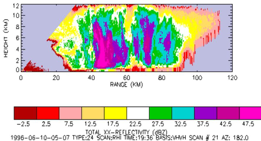
An example of a weather radar signature of a 'killer' rainfall rain event recorded with a modern Polarimetric-Doppler. Such information can potentially save lives.
